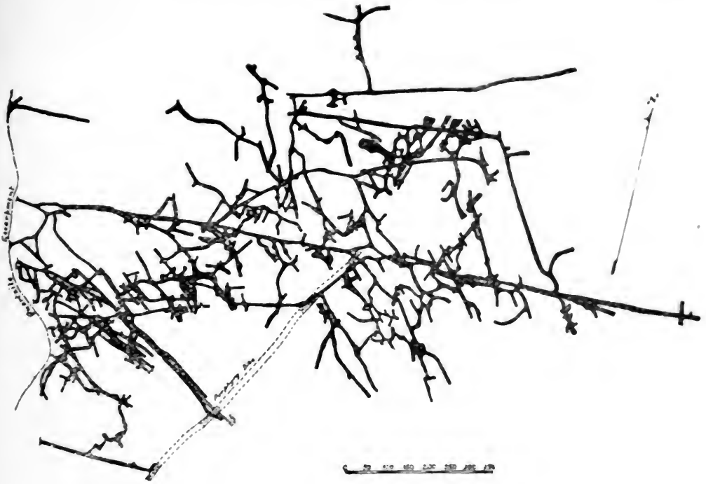
FIG. 17.—The drifts follow the lines of fissure as shown in the section in Fig. 16. The mine workings thus bring out clearly the fissure systems.
